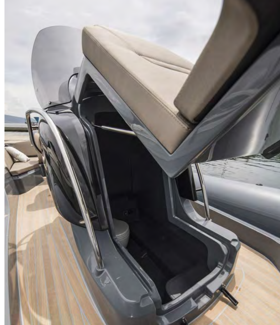
Toilet under console
